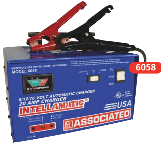
Model 6058 20 Amp 8/12/16 Volt Smart Charger Rocker switch is used to select battery size 8V for monoblock batteries – used on many golf carts 12 V standard batteries 16 V high performance batteries
